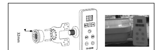
install at left or right side of the instrument tray box, adjust direction 180  $^{\circ}$
